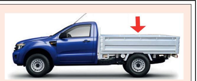
Some flat-deck pickups (like the one above) have removable sides that can be fitted around the deck to form an enclosed tray.
